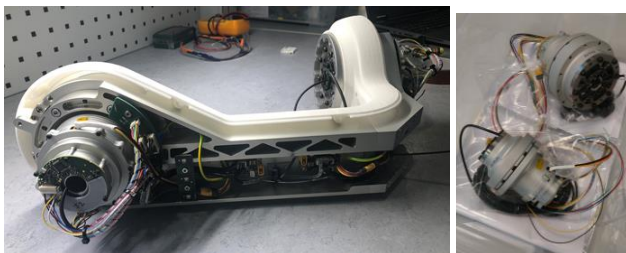
Figure 4: X-ARM hardware integration. Link 1 (left) and small and heavy duty joints (right)
