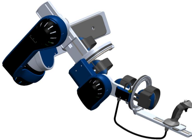
Figure 3: X-aRm exoskeleton. Technology demonstrator with 3 active degrees-of-freedom and 2 sensorized joints.
