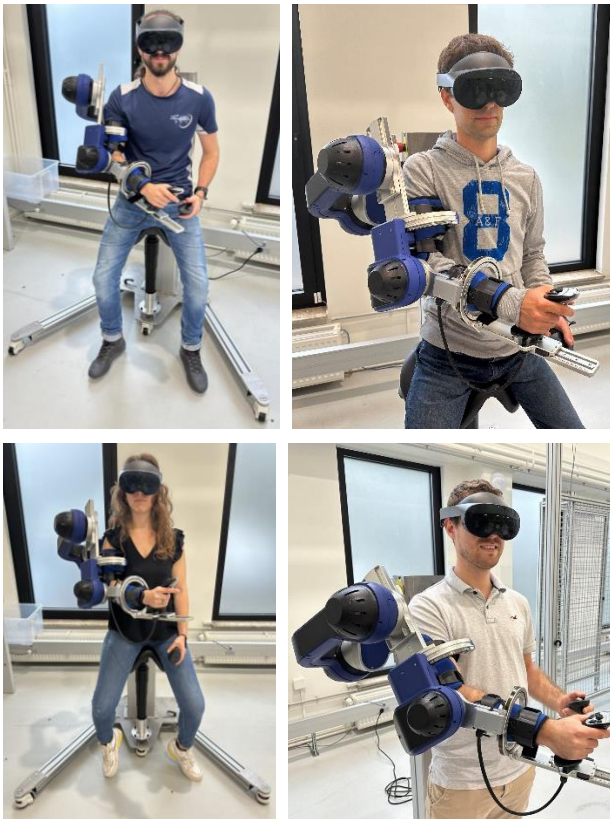
Figure 7: Integrated X-aRm system with different candidates validating comfort, adjustability and portability.
